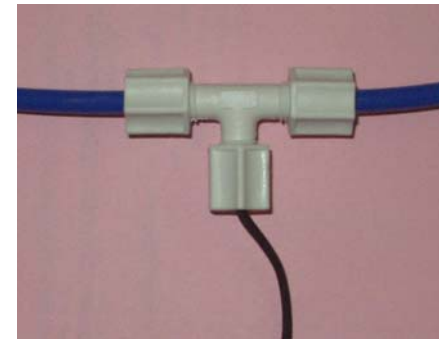
Fig. C: In-Line Probe Location
